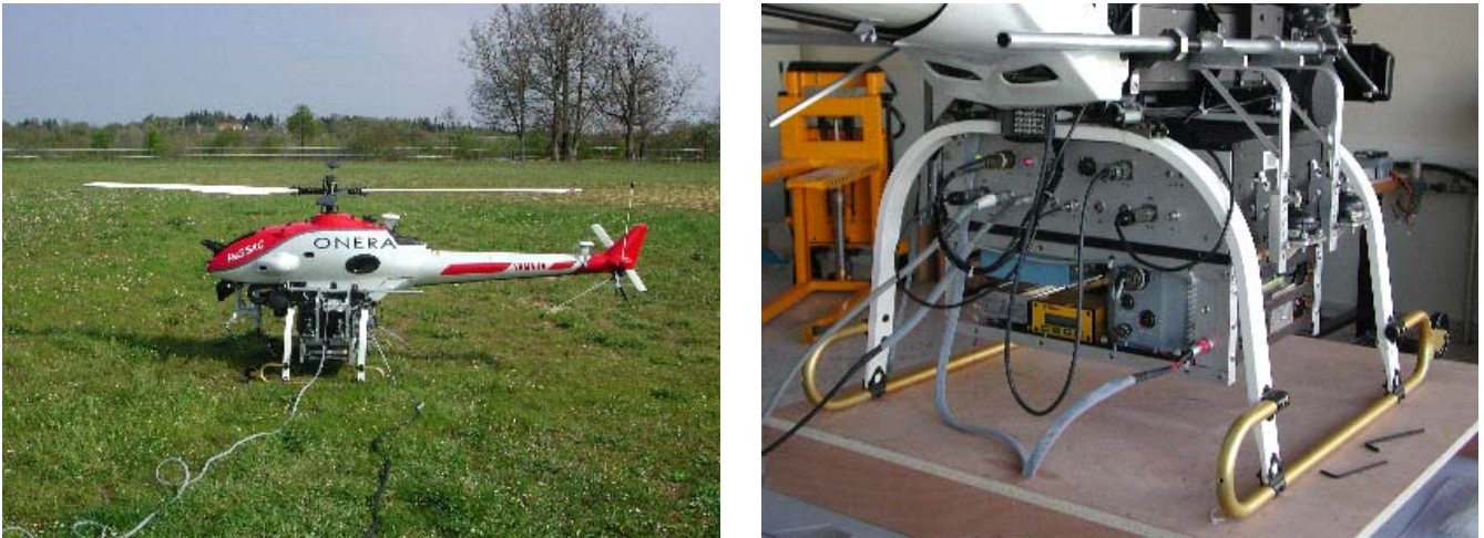
Figure 5: Tests with a real UAV; integration of the shipborne segment on the R-MAX RESSAC UAV of Onera
