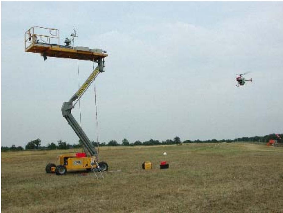
Figure 7: Tests on a real UAV with the decking platform physical simulator (simulator located at 7 m above the ground; laser sheets not visible in day light)
